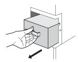
**6.** Carefully insert the new lamp unit straight into the TV until it is fully seated. The lamp unit is fully seated when the two plastic "nubs" on the TV cabinet are flush with the two holes in the lamp unit (above and below the lamp unit screw hole; see illustration below).
